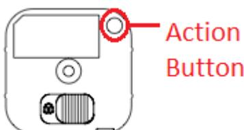
3. If your MultiSensor has been successfully removed from your network, the RGB LED will be active with a colourful gradient for 3 seconds.
