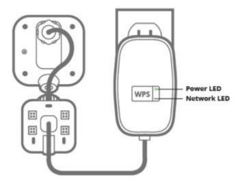
**Note**: Please ensure that the camera is paired to your network before permanent mounting. The PoE power adapter is for indoor use ONLY. It is not weatherized for outdoor placement.
