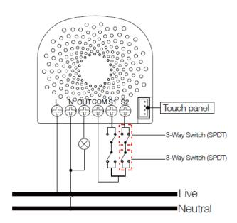
You may follow the article <u>Nano Dimmer wiring 3-way/4-way/5-way switch methods</u>
