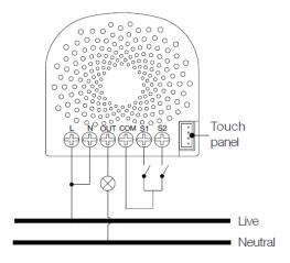
Note: The "N" terminal should be connected to the "L" terminal when the Nano Dimmer is installed by 2-Wire system.
