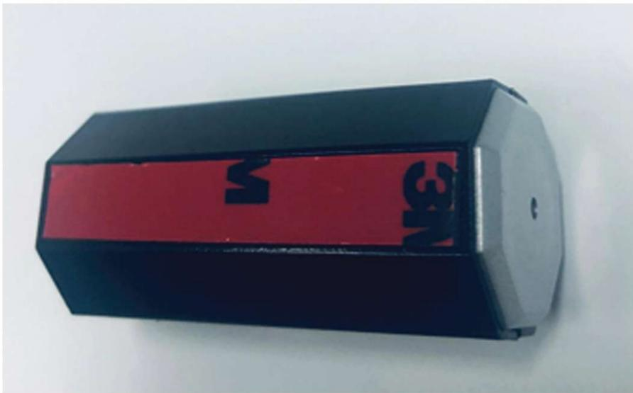
**Step 2:** After installing the Octagon, the distance between the two components of the sensor should be less than 10mm when the door/ window is closed. For the sensor to trigger an alert, the separation between the two components should be over 20mm (for open status )and less than 10mm (for close status )
