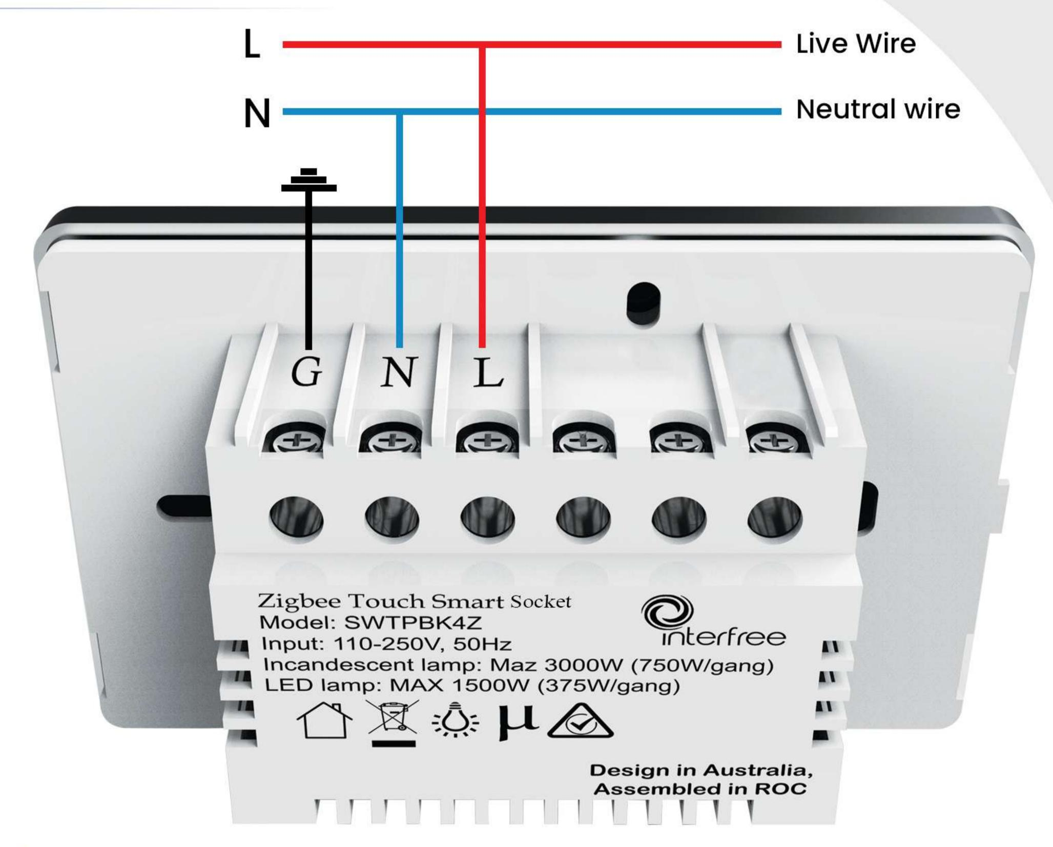
Please wire up the switch strict accordance with the diagram in the prevention of any damage to the switch. This product must be installed by a qualified electician.
