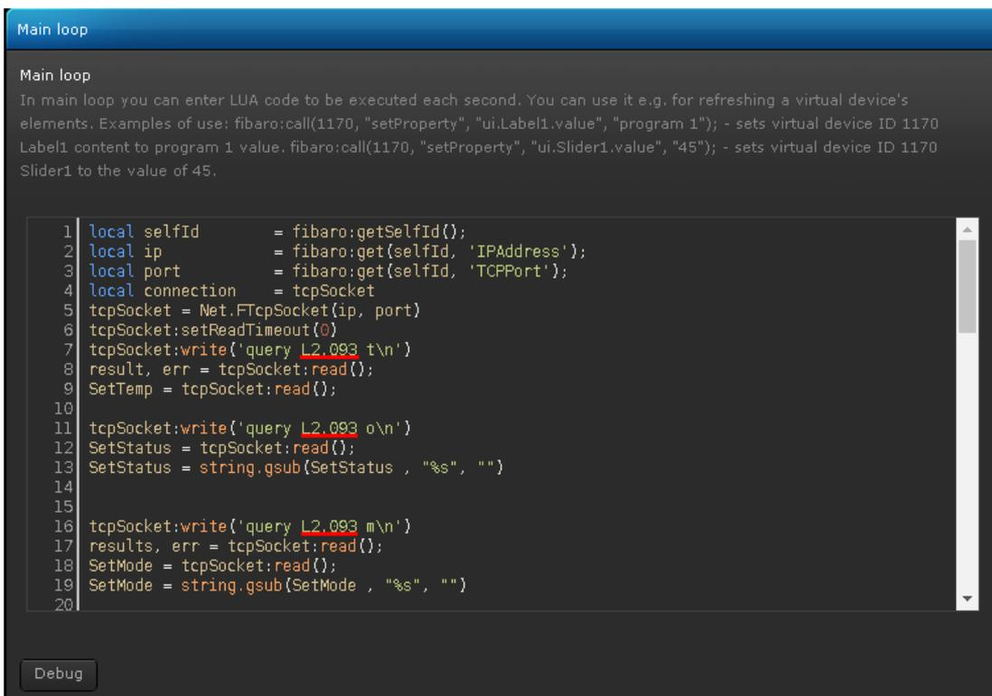
Once you have changed all noted **L2.093** you will need to scroll back up and save the Virtual Device, once you have done so you will be able to control the CooLinkHub, and as long as you have done it all correctly you will also receive feedback from your HUB so if you change the Temperature manually the Remote will also update the temperature on the FIBARO HC.
